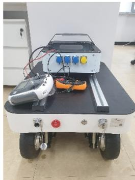
Fig.1: Ackermann based mobile robot
